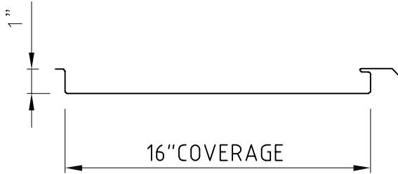
Soffit Profile (Flat Pan Standard)
