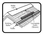
Always check the corrugated sheets and closure strips for proper fit. Closures may come with adhesive, should match sheet profile, and must be compatible with polycarbonate.
