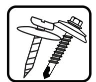
Fasteners should penetrate the roof or wall of the structure by at least one (1) inch. A 1/2" neoprene bonded washer is recommended for most applications. If aesthetic concerns arise, a smaller washer may be used if it provides a flat bearing surface and creates an effective seal.
