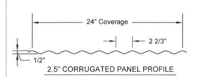
Panel Fastener Side Lap Fastener 2.5" CORRUGATED PANEL SEAM
