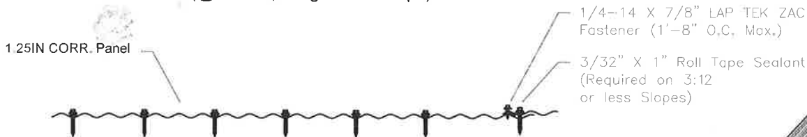
FASTENER PATTERN (@ Intermediate Purlins)
