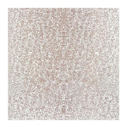
Galvanized G90. Material is sold with no warranty. The sample shown here has a mid to large spangle design but can vary from run to run. Galvanized is initially shinier then Galvalume but weathers to a duller appearance over time.
