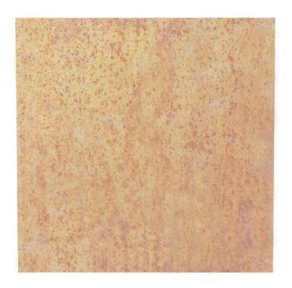
Cold Roll steel. This material is intended to rust. It has no rust inhibitors such as zinc or aluminum so it requires no preparation when a rusty appearance is desired. This material is typically run in heavier gauges (thicker material) to detour from penetration by rust.
