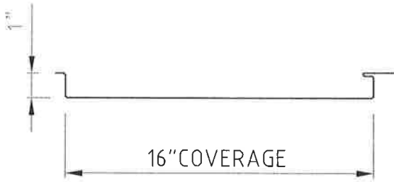
Soffit Profile (Flat Pan Standard)
